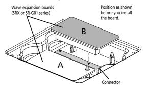
The slot you choose is of no importance. Be aware, however, that there are two expansion sound groups ("A" and "B") and that the slot you choose here specifies which group you need to select on the front panel. (4) Use the installation tool supplied with the wave expansion board to turn the holders in the LOCK direction, so the board will be fastened in place.
